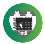
The last black dot on the matrix indicates the correct temperature. After the initial reading, all future readings are available instantaneously for a continuous 48-hours.
